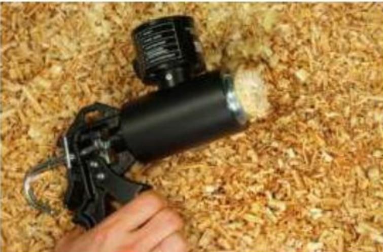
7. After doing so, pull back the compacting device and close the head again.
