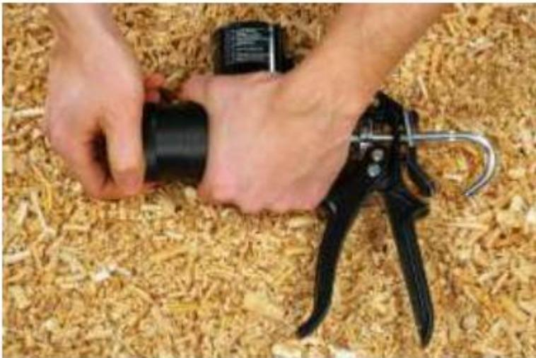
2. Pull back the compacting device completely in order to ensure that the measurement chamber can take the maximum volume.
