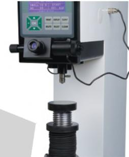
**Note: The eyepiece should be completely inserted in to the sleeve, otherwise, the measurement will be not accurate.**
